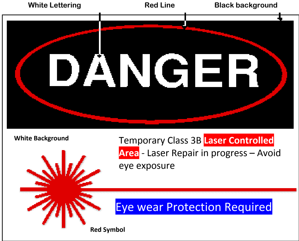
Figure 4 – Temporary Warning Sign requiring immediate hazard recognition
